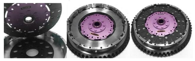
8) Mount the main pressure plate casting into the adapter ring with the fulcrum facing up. Then mount the alloy cover to the adapter ring
