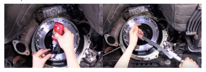
5) Apply a small amount of spline grease to the spline on the clutch disc and slide it onto the input shaft rotating it several times. Wipe the excess build-up off the edge of the hub and repeat with the other disc.
