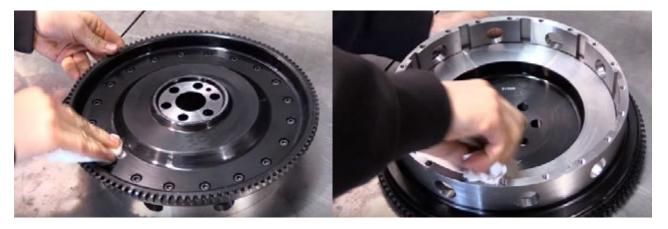
4) Use thread locking compound on the flywheel bolts and torque to manufacturers specifications.
