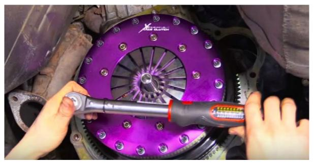
11) When the 10 M6 bolts have pulled the alloy cover up to the adapter ring firmly the remaining 10 pressure plate bolts can be installed. At this point torque all 20 bolts up to 13ft.lbs/ 18N.m.
