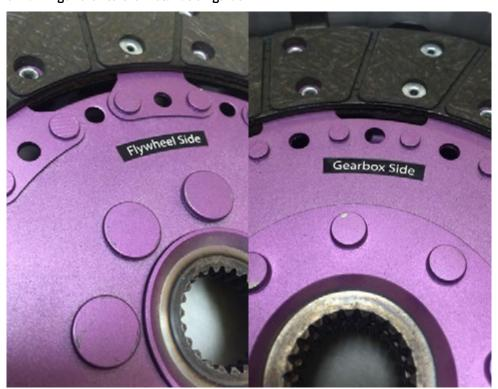
Install the flywheel side friction disc followed by the intermediate plate and then the transmission side friction disc ensuring that all parts are clean and that the orientation is correct (facing with "flywheel side" sticker must face the flywheel and facing with "gearbox side" must face the clutch cover. At this point use the alignment tool to align the friction discs to the pilot bearing.
