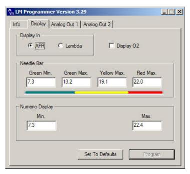
The MTX-L gauge can be setup to display different ranges from both the Needle Bar and the Numeric Display. There is also an option to display lambda or AFR. Lastly, the gauge can be setup to display percentage of Oxygen once the readings go beyond 7 lambda.
