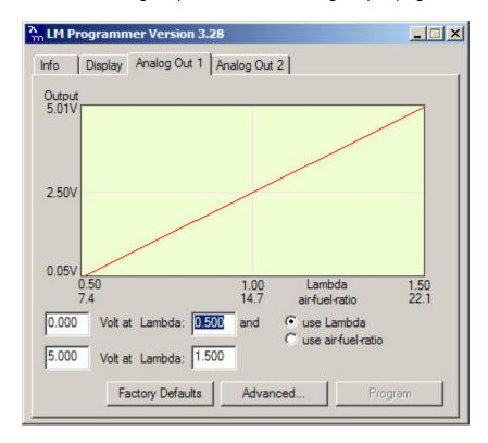
This shows the analog output voltages versus Lambda for one of the two analog outputs. The graph display is automatically scaled to the selected voltages. For each output you can specify a minimum and maximum lambda value and the associated voltages. Below the minimum and above the maximum lambda values the output voltages stay constant at the associated programmed voltage.
