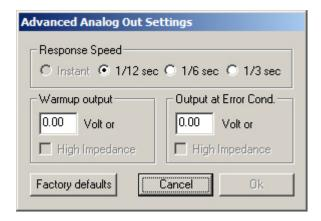
When setting the MTX-L to the slower response speed settings the measured mixture data will be averaged over the response time setting before being output.
